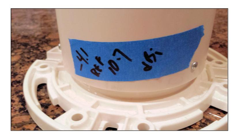
FOUR WHEEL ARRAY: 10.7 - 4.1 = 6.6 dBi GAIN
